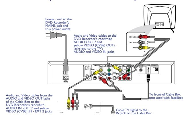
Your Cable Box may have Audio and Video Out jacks instead of a single ANTENNA OUT, TO TV, or RF OUT jack as shown on page 2 of this Guide. If so, use the Audio and Video Out jacks to connect the Cable Box to your DVD Recorder.
