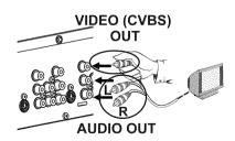
Switch on the TV. Then switch the TV to the Video/Audio input jack or select the corresponding channel number. For the channel number, please see your TV's instruction manual.
